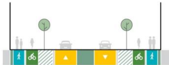
Figure 5: Proposed Cross Section of Roading Upgrades (24m) in the vicinity of the Submitter’s site.
