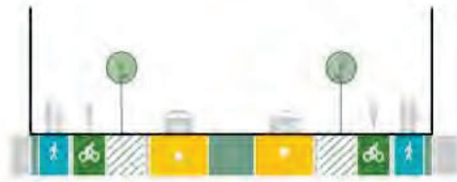
Figure 5: Proposed Cross Section of Roading Upgrades (24m) in the vicinity of the Submitter’s site.
